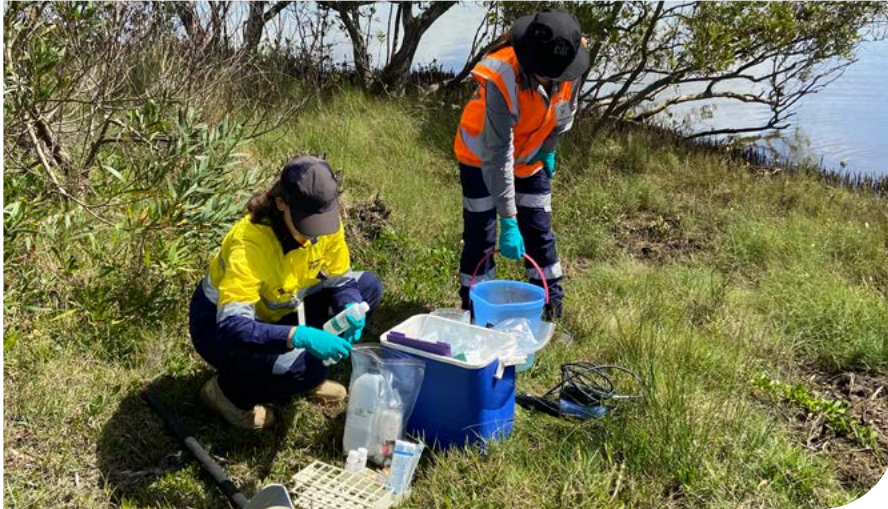
Samples collected at Lake Macquarie are put into an esky with ice for immediate delivery to the lab. Photo: EPA
