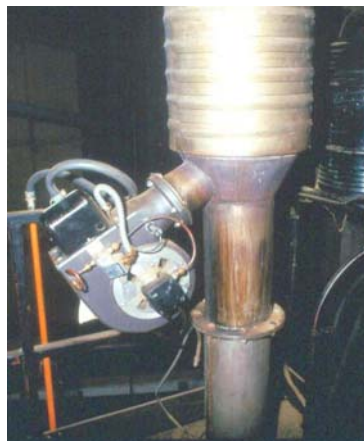
A small afterburner for rendering odours
