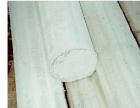
Pulse jet bags showing bottom closure
