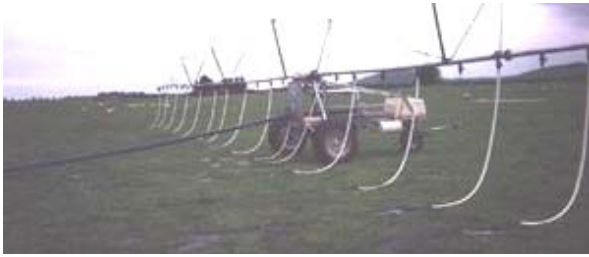
Travelling effluent irrigator with droppers
