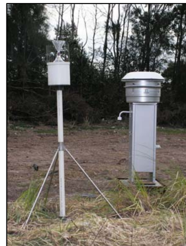
Simple air pollution monitors on a large construction site
