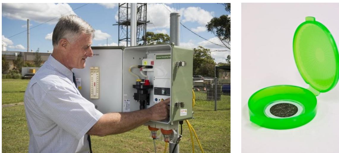
Figure 3-1. Left: ASP PM 2.5 cyclone sampling unit at Lucas Heights site. Right: An exposed 25mm stretched Teflon filter in its container. Photos: C Thompson/ANSTO
