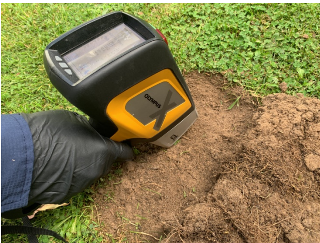
Figure 1 Screening soil at Captains Flat with an XRF analyser. Photo: David Langston/EPA.
