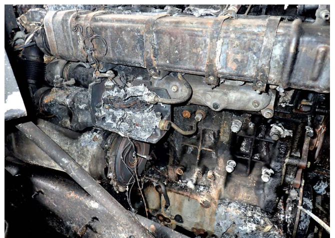
An engine bay after a fuel fire.
