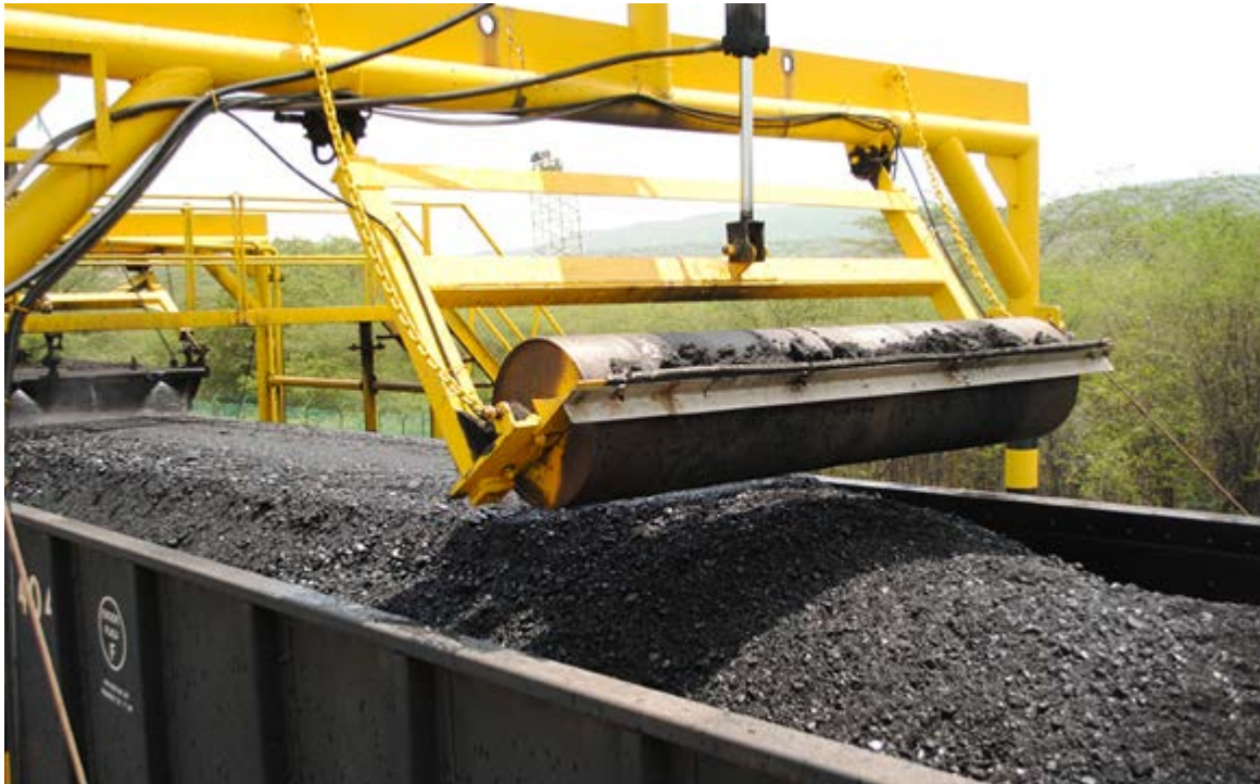
Figure 14 Coal wagon compaction at Cerrejon Mine in Columbia (Source http://www.cerrejon.com )
