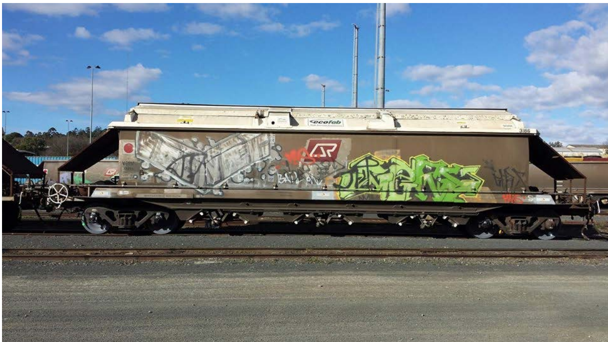
Figure 15 Retrofitted lid on an old coal wagon now used for grain transport
