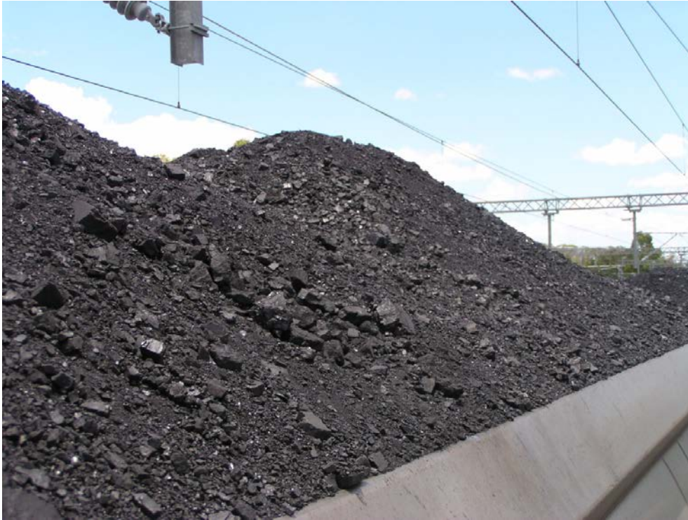
Figure 11 Photograph showing a poorly loaded wagon (extracted from Connell Hatch, 2008)
