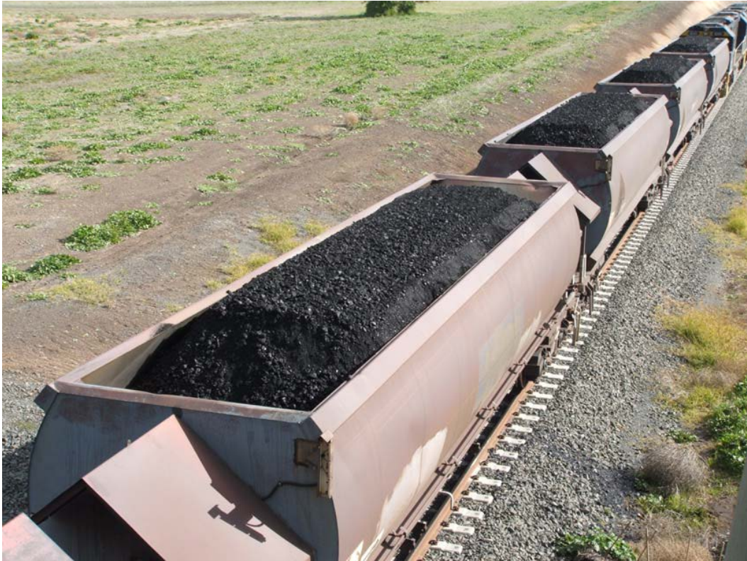
Figure 8 Typical open topped coal wagon used in Queensland (Connell Hatch, 2008)
