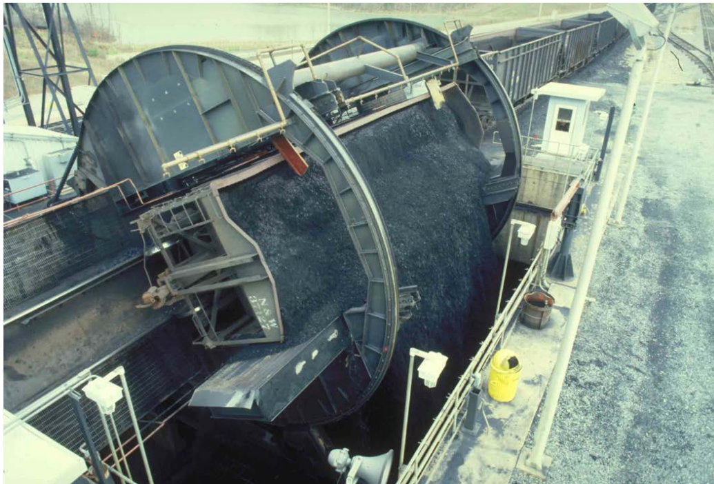
Figure 17 Rotary dump unloading
