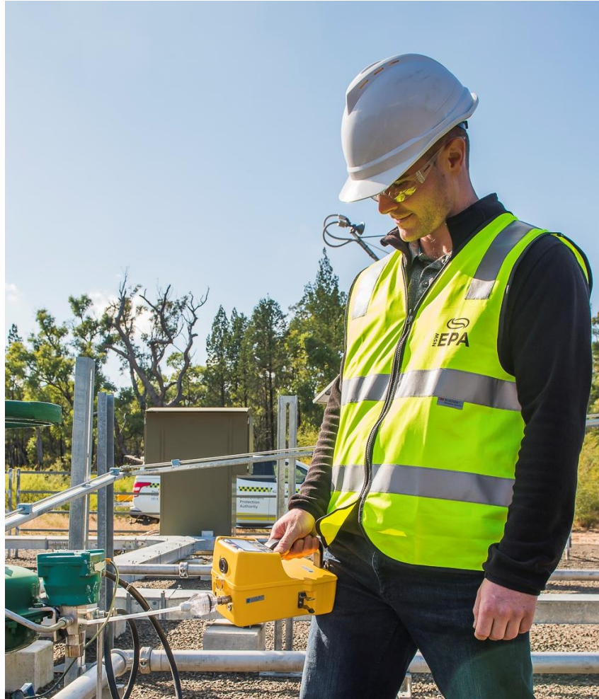
Picture: An EPA operations officer holding the Eagle 2 gas monitor
