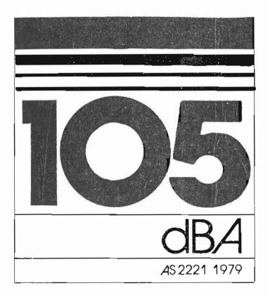
4.2 Mobile Air Compressors - The Mean Sound Level of a unit shall be displayed on a label with dimensions 9 cm x 10 cm. Format, lettering and numbering size shall, as far as practicable, be identical with the relative scale of the format, lettering and numbering size given in the following example:
