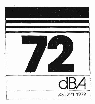
4.3 The labels for both pavement breakers and mobile air compressors shall have a permanent clearly visible black legend on a white background.
