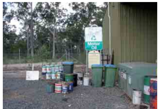
Photo 37.9 Collection of waste oil (Note: Waste oil and other liquid wastes should be stored in a covered and bunded area)
