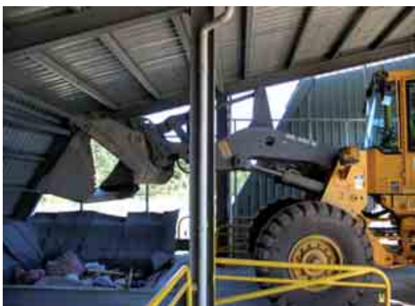
Photo 30.8 Compaction of mixed waste using site plant
