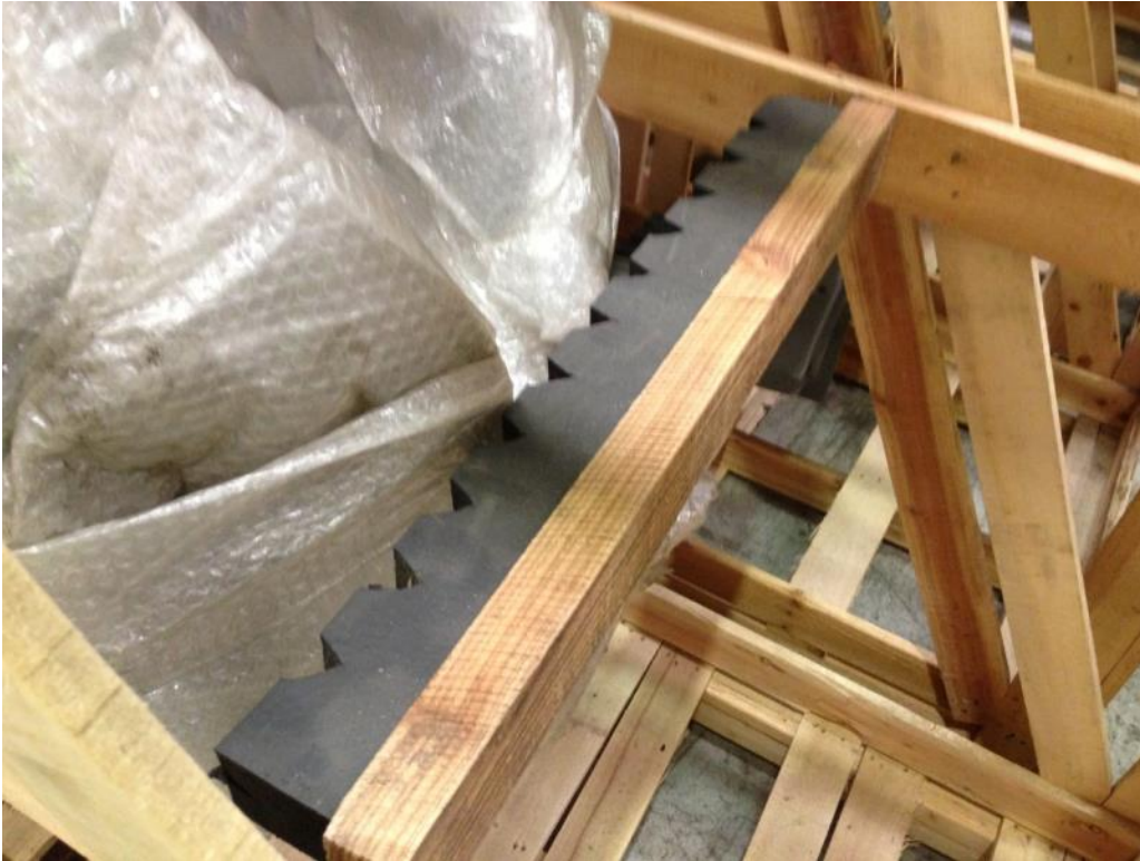
Photograph 7: Packaging – mix timber/metals/foam – timber not recycled as metal/foam considered as contamination. Is not separated at site level due to labour required
