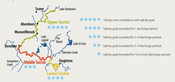
Salinity is measured by determining the electrical conductivity (EC) of water, EC estimates the amount of total dissolved salts in the water, and is measured in microSiemens per centimetre ( $\mu$ S/cm). Saltwater has an EC of around 55,000  $\mu$ S/cm. Drinking quality water usually has an EC of between 600 and 1200  $\mu$ S/cm.
