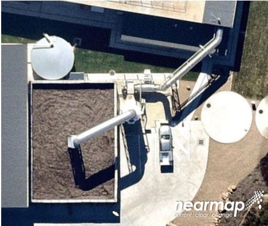
Figure 22 Aerial view of a biofilter treating odour ducted from a building Source: Nearmap aerial image
