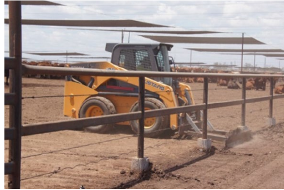
Figure 3 Cleaning manure under fences Source: Tucker et al. 2015
