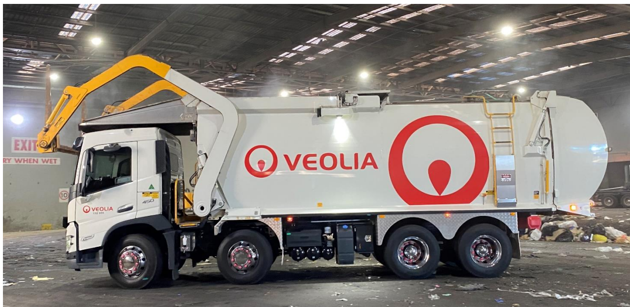
Image 11 Front-lift vehicles were the most common mode of delivery at both landfills and transfer stations Credit: APC Waste Consultants
