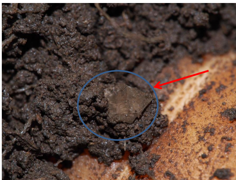
Plate 3b. Visible glass in soil adhered to carrots harvested from glass amended soil
