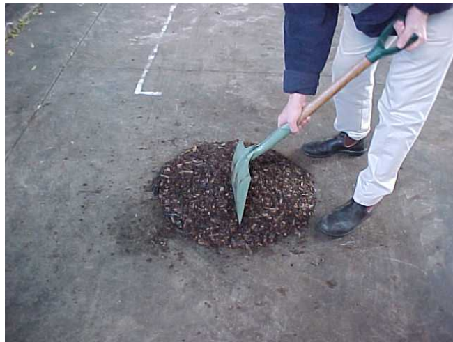
Plate 3. Sub-sampling of the combined sample by coning and quartering. The combined sample is formed into a cone, and divided into quarters.
