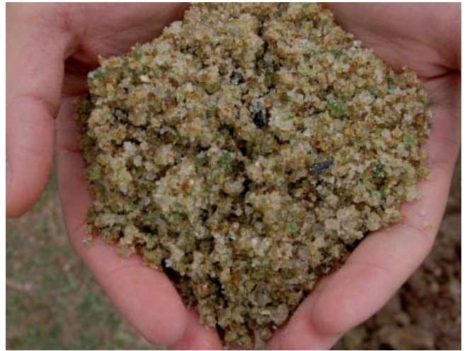
Crushed recycled glass used in the trials
