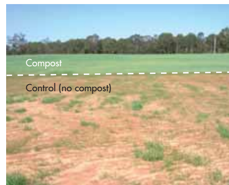
Figure 2 Photo of the trial three months after construction. Note the poor turf establishment and erosion occurring in the control area (foreground), and the very good turf establishment where compost was applied (background).
