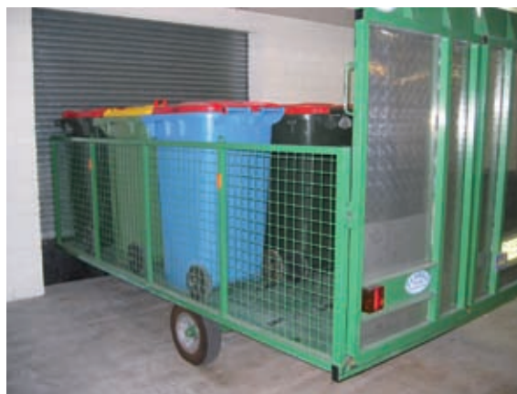
Trailer used to move bins from intermediate to central storage and collection area
