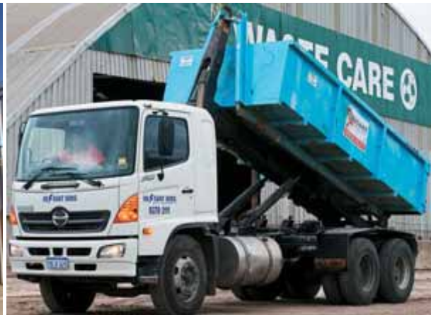
(c) Bulk bin serviced by hook lift
