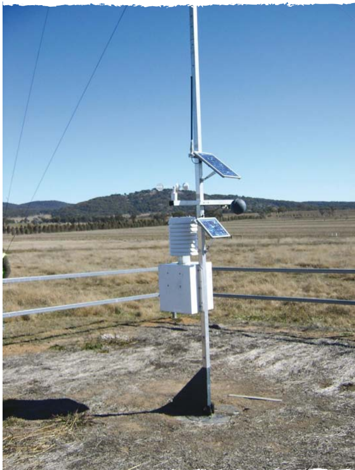
A solar-powered automatic weather station provides site-specific, accurate and continuous monitoring of weather data to inform decisions on effluent irrigation (photo: W Wickremeratne/DECCW)
