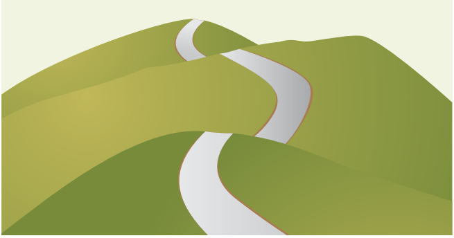
Figure 5.2: Mid-slope road with a side cut
