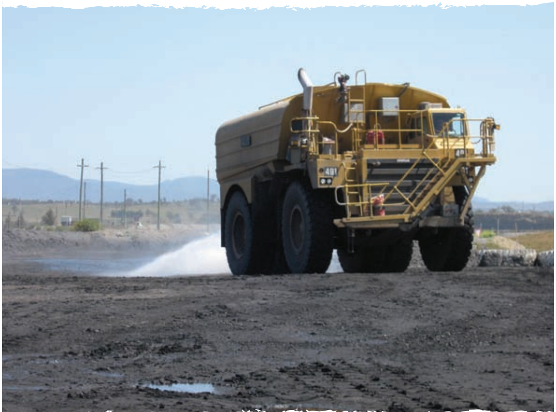
Water carts are often used to help suppress dust from haul roads (photo: J Pope/DoP).
