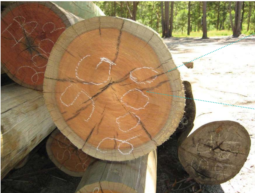
Figure 3: Preservative treated sapwood - apparent in cross-section
