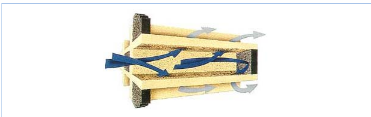
Figure 6-5: Schematic of wall flow DPF monolith structure
