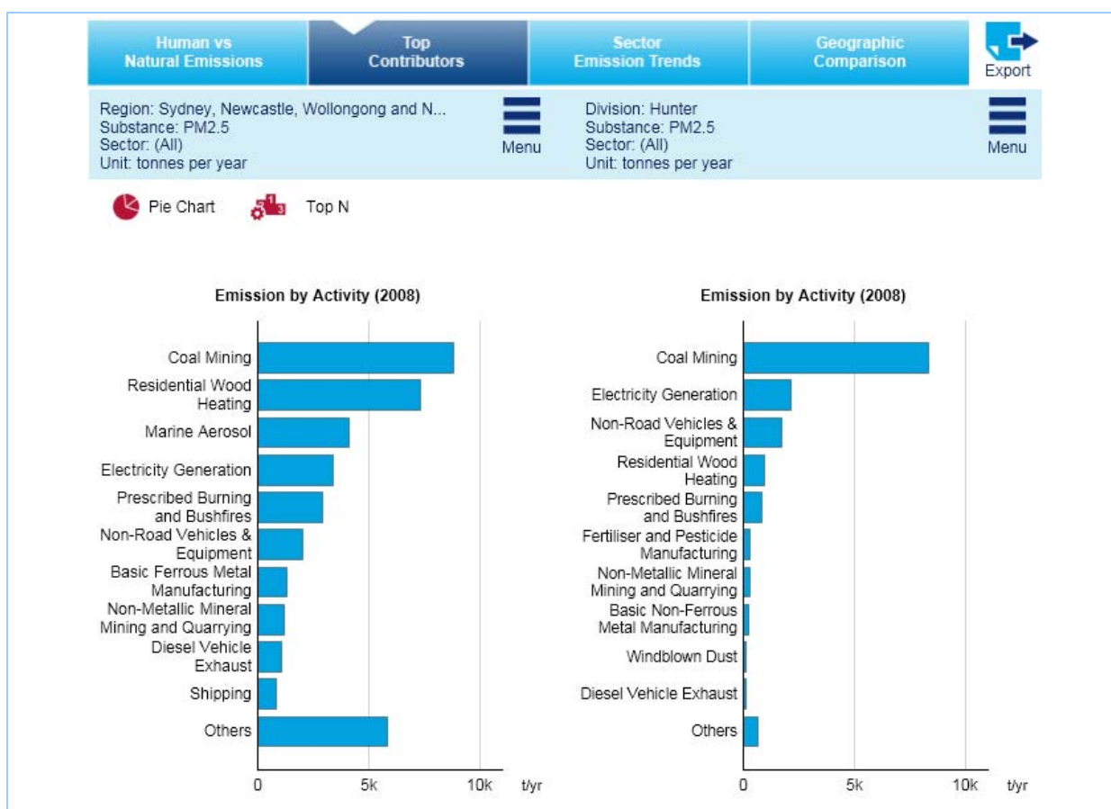
Figure 3-5: Top 10 sources of primary PM 2.5 emissions in the GMR and Hunter region
