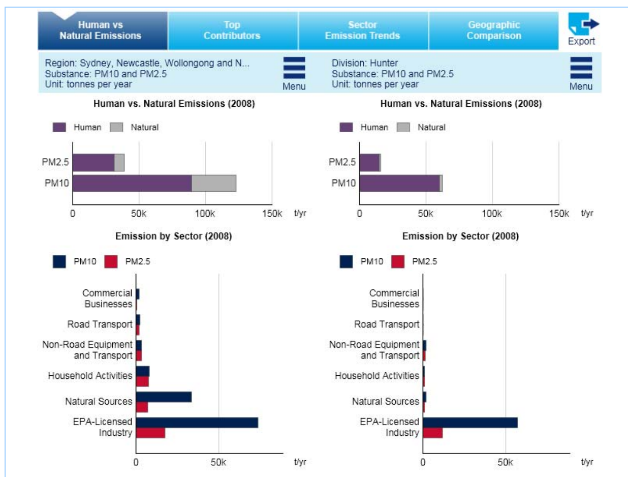
Figure 3-3: Natural vs. human-made emissions of primary PM 10 and PM 2.5 in the GMR and Hunter region
