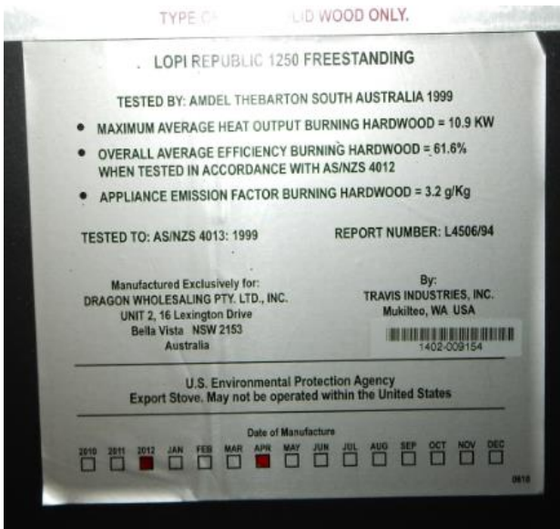
Figure 2: Wood heater appliances with particulate emission factors greater than 2.5 g/kg (Photo: Karin Schianetz, EPA)
