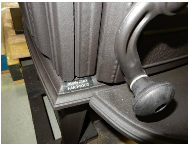
Figure 9: Fuel type plates not considered permanently attached and legible (Photo: Aleksandra Young, EPA)
