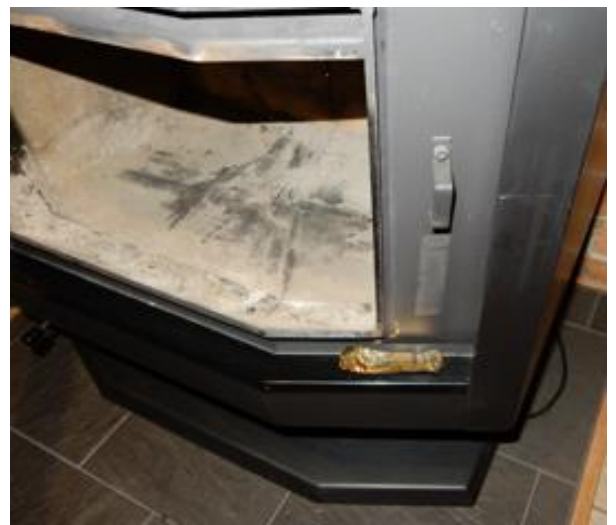
Figure 10: Fuel type plates where the wording is not visible after short use of wood heaters (Photo: Antonia Curcio, EPA)
