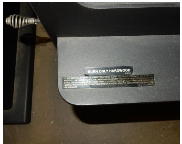
Figure 9: Fuel type plates not considered permanently attached and legible (Photo: Aleksandra Young, EPA)
