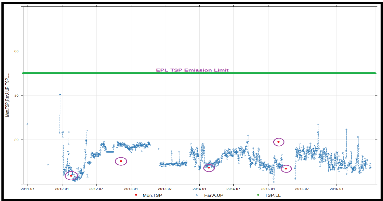
Figure 10: Eraring Unit 1, Duct A - Daily average of Opacity CEM, as undifferentiated particulates and stack test TSP ( \text{mg}/\text{m}^3 )
