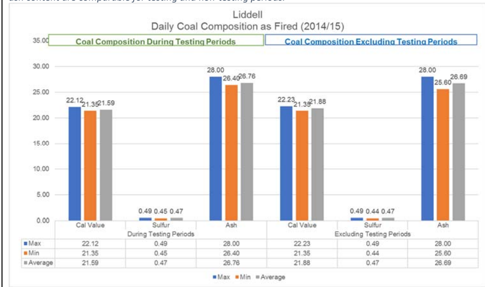
Figure 34: Liddell Daily Coal Composition as Fired (2014/15) showing the average calorific value, sulfur and ash content are comparable for testing and non-testing periods.
