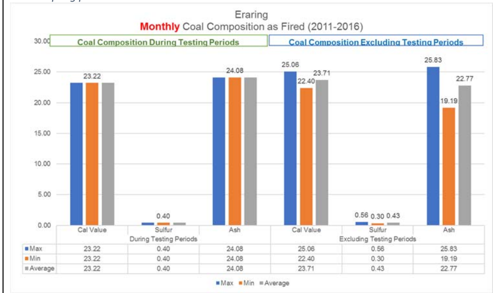
Figure 39: Eraring Monthly Coal Composition as Fired (2011-2016) showing the average calorific value, sulfur and ash content are comparable for testing and non-testing periods. Note: Coal Analysis data is only available on a monthly basis. Coal composition data is only representative of one sampling period.
