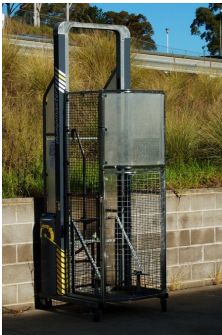
Examples of bin-lifting devices
