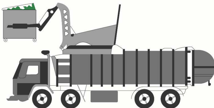
Front-lift-loading waste collection vehicle
