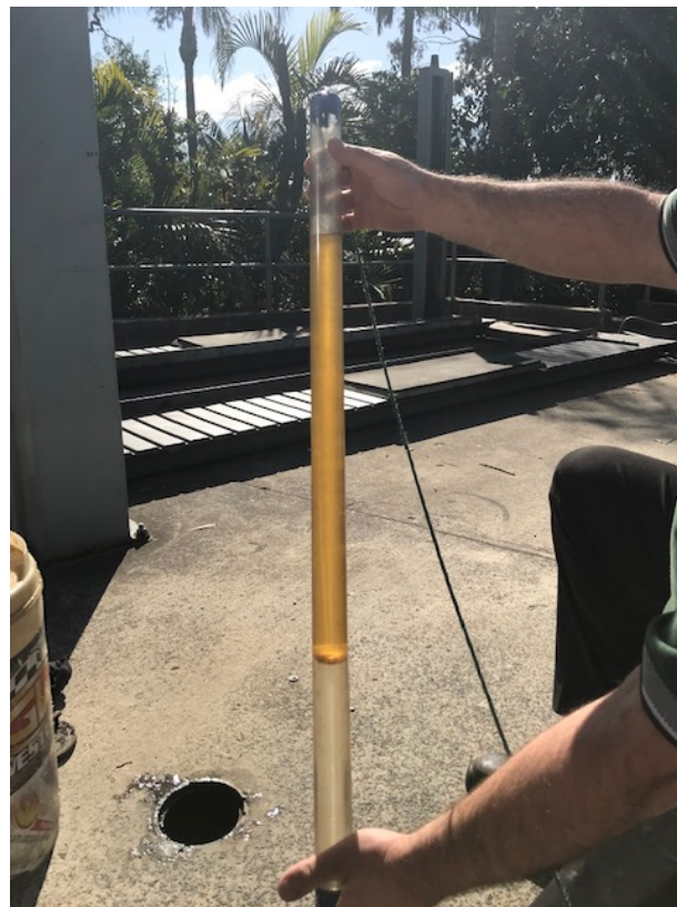
Image 2: groundwater monitoring showing fuel contamination in the groundwater
