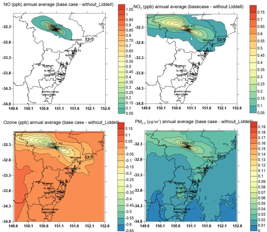
**Figure 3** Difference in simulated annual average of NO, NO<sub>2</sub>, O<sub>3</sub> and PM<sub>2.5</sub> between base case and S1 scenario as predicted by CCAM-CTM model over the GMR in 2013
