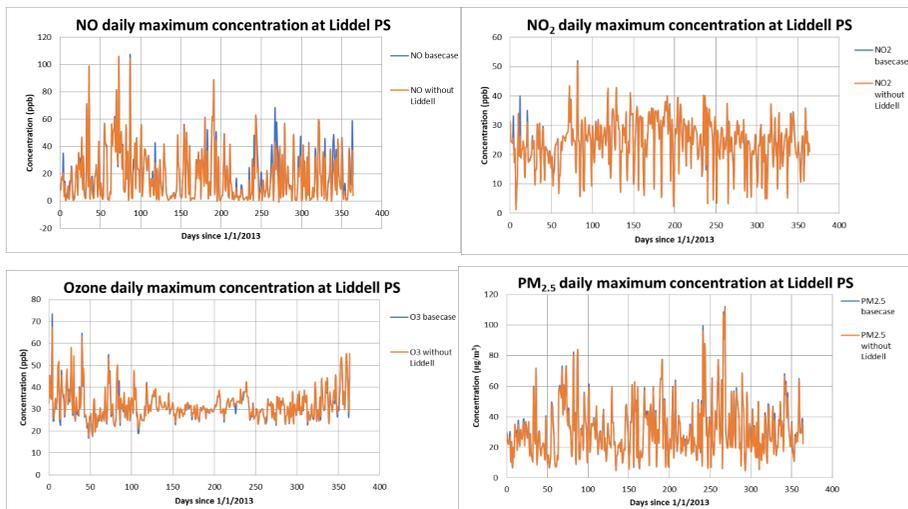
**Figure 7 Plots of predicted daily maximum NO, NO<sub>2</sub>, O<sub>3</sub> and PM<sub>2.5</sub> concentrations at LPS for 2013 from the base case and S1 scenario simulations.**
