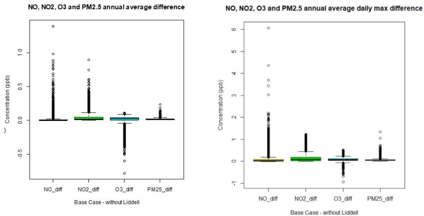
**Figure 4** Box plots of differences in annual averages (left) and annual average daily maximum levels in the GMR domain between the base case and S1 scenarios for NO, NO<sub>2</sub>, O<sub>3</sub> and PM<sub>2.5</sub>
