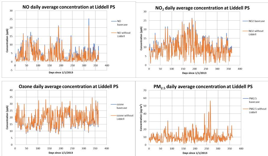
**Figure 5** Plots of predicted daily average NO, NO<sub>2</sub>, O<sub>3</sub> and PM<sub>2.5</sub> concentrations at LPS for 2013 from the base case and S1 scenario simulations.
