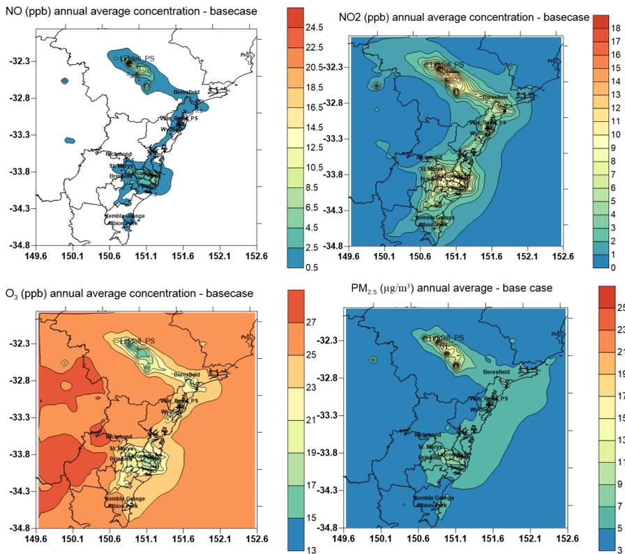
**Figure 2 Annual average of NO, NO<sub>2</sub>, O<sub>3</sub> and PM<sub>2.5</sub> as predicted from CCAM-CTM over the GMR in 2013 – base case**
