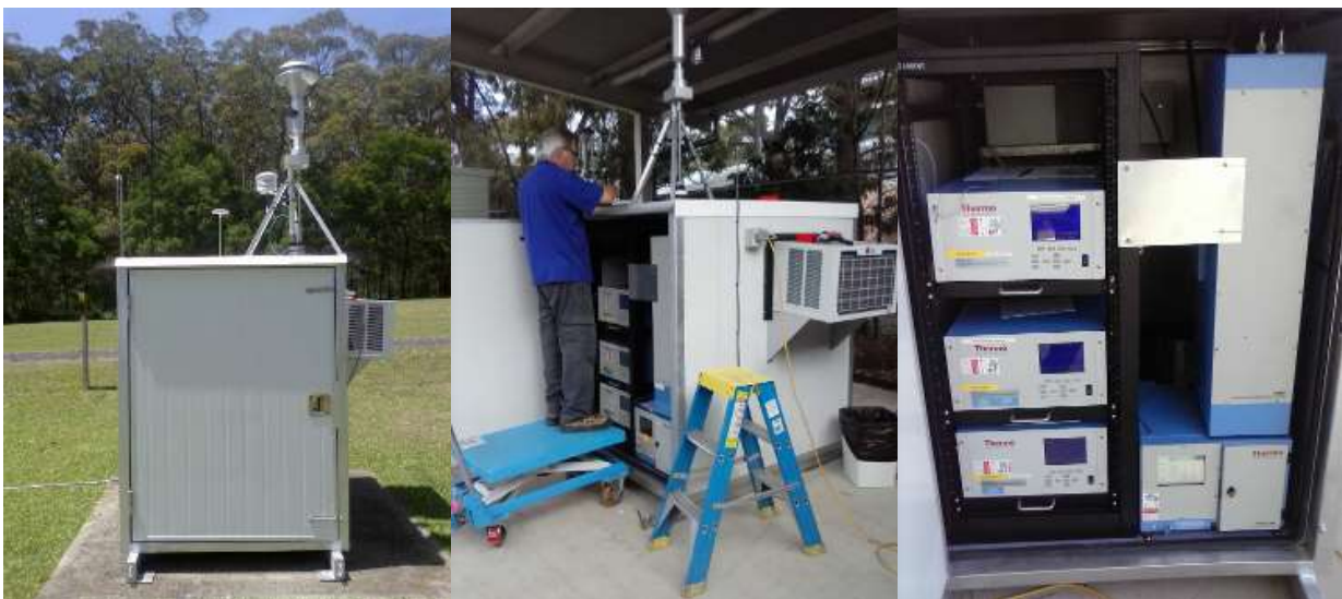
Figure 45: OEH portable monitoring station able to hold up to seven air quality monitors that comply with Australian Standards and with the AAQ NEPM
