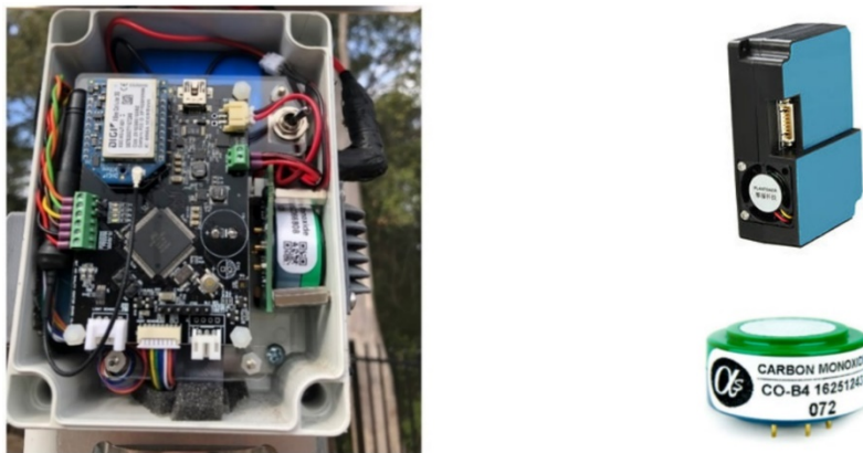
Figure 4: KOALA fitted with Carbon Monoxide and Particulate Sensors
