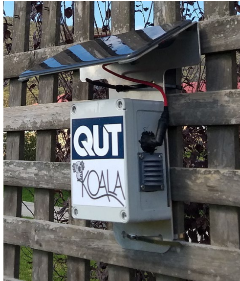
Figure 1: KOALA low cost air monitoring sensor (QUT)
