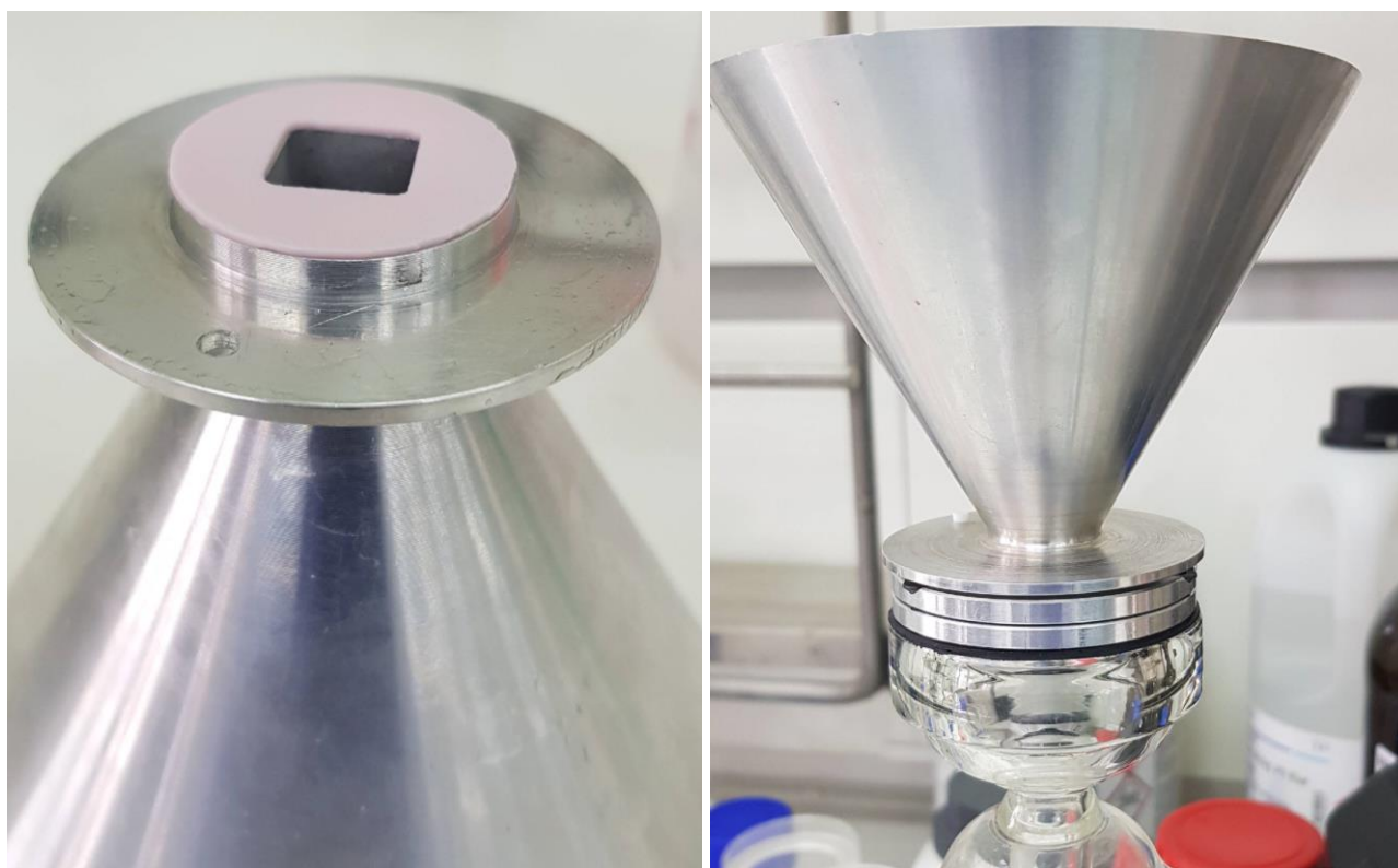
Figure 3 Filtration apparatus for mounting Anodisc filter for final filtration of collected particulates.
