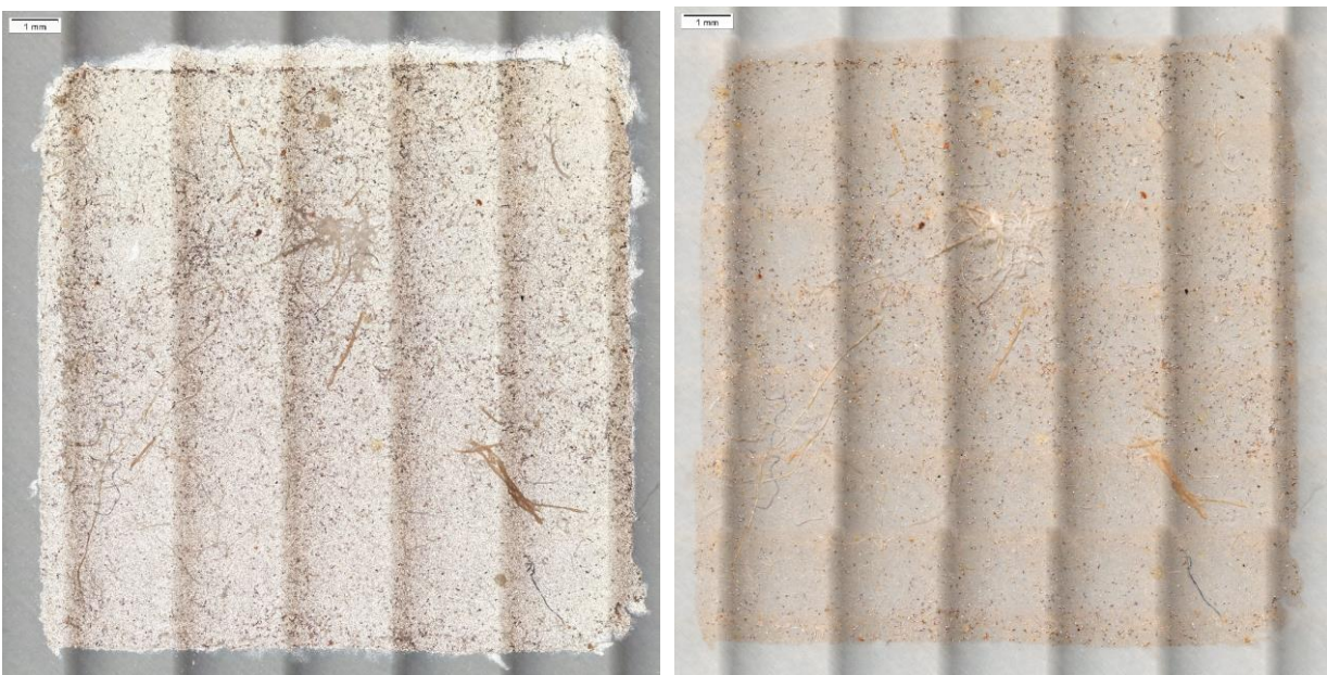
Figure 4 Representative brightfield (L) and dark field (R) optical image of material collected onto an Anodisc filter. The vertical dark lines are artefacts of stitching many images with non-uniform illumination together.
