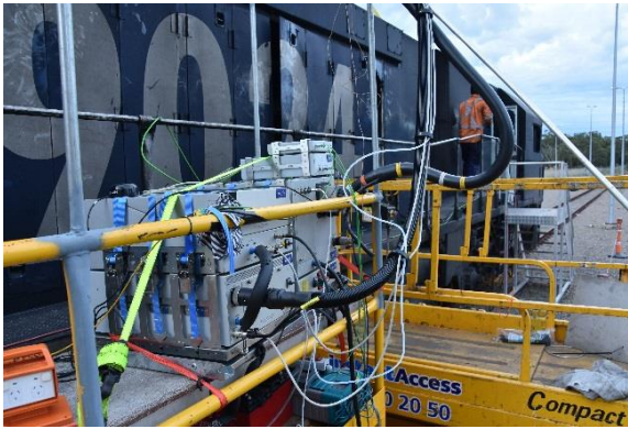
PEMS setup with emissions sample lines (example)
