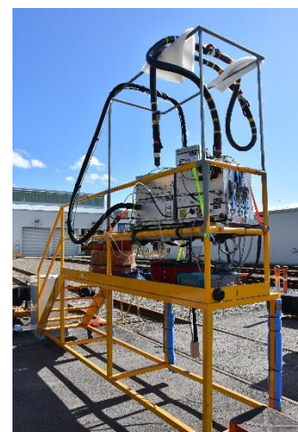
PM and Gas PEMS set up prior to the locomotive arriving
