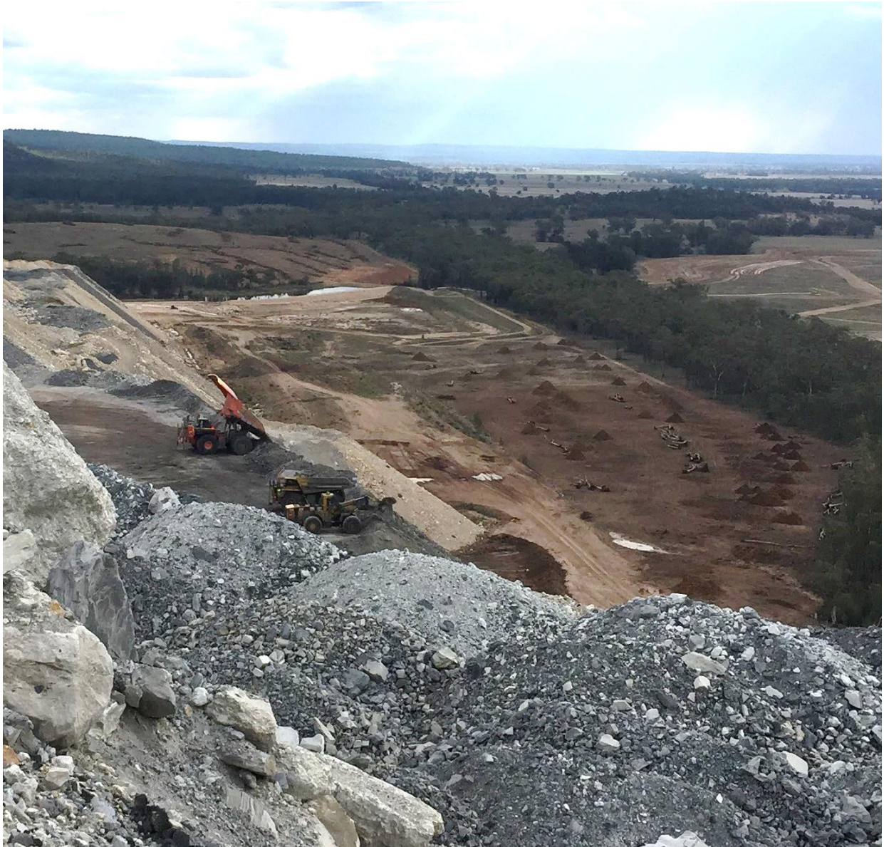
Figure 21 Truck dumping overburden on northern overburden emplacement of MCCM
