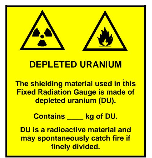
D7 Example of a Suitable Warning Label for Attachment to a Shutterless Fixed Radiation Gauge
