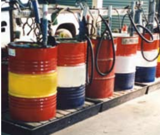
Bulk liquids used in the workshop should be kept in a bund.
