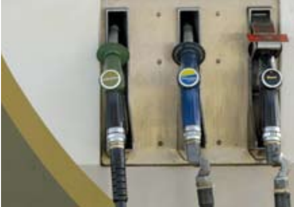
Make sure fuel pump nozzles cut off automatically when the tank is full.
